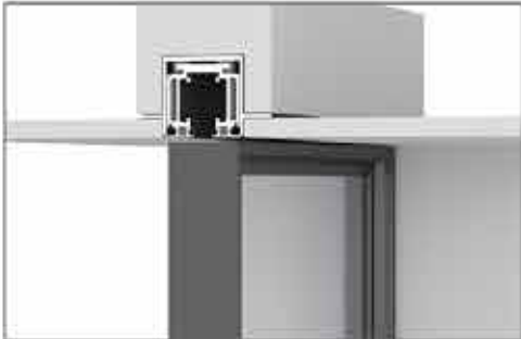
Monorail Shock Absorbing Track Track dimensions: 47.8*87.8
